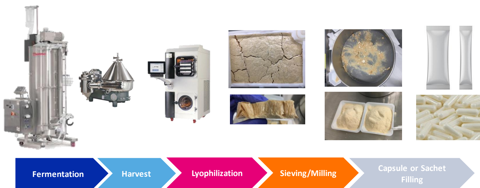
Figure 2. Process to develop a solid SYN1618 formulation
